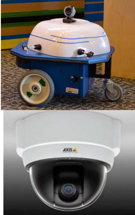
Figure 1. Robotic platform used in stationary and mobile conditions, wall-mounted pan-tilt-zoom camera.
