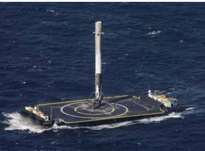
SpaceX's innovation in rocket reusability offers the possibility of more affordable access to LEO and beyond. Here, its Falcon 9 rocket lands after launching. (SpaceX)
